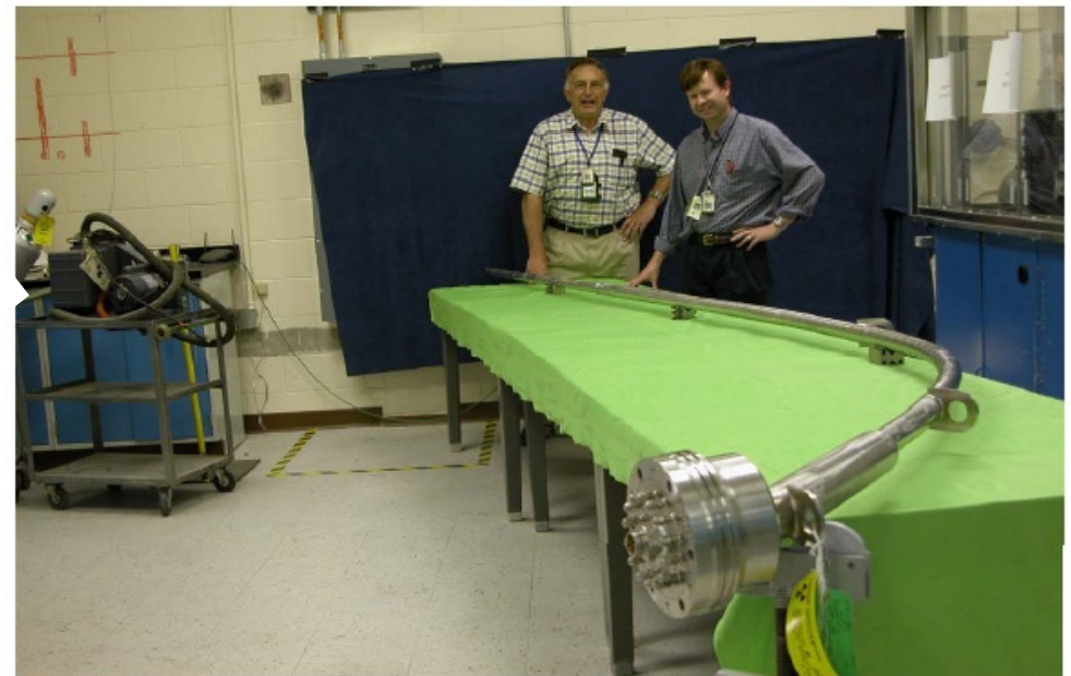
AGR-1 test train assembly 6-individual instrumented capsules
